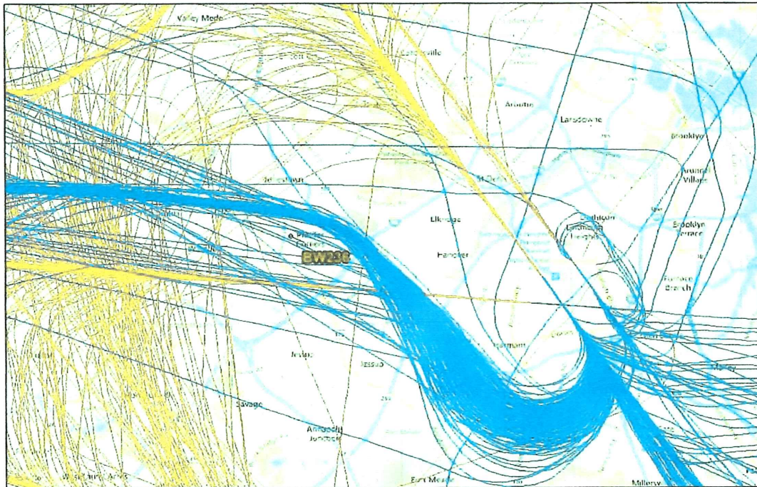
Figure 5. All Flight Tracks for an East Flow Day – March 13, 2016 (red = arrivals, blue = departures)
