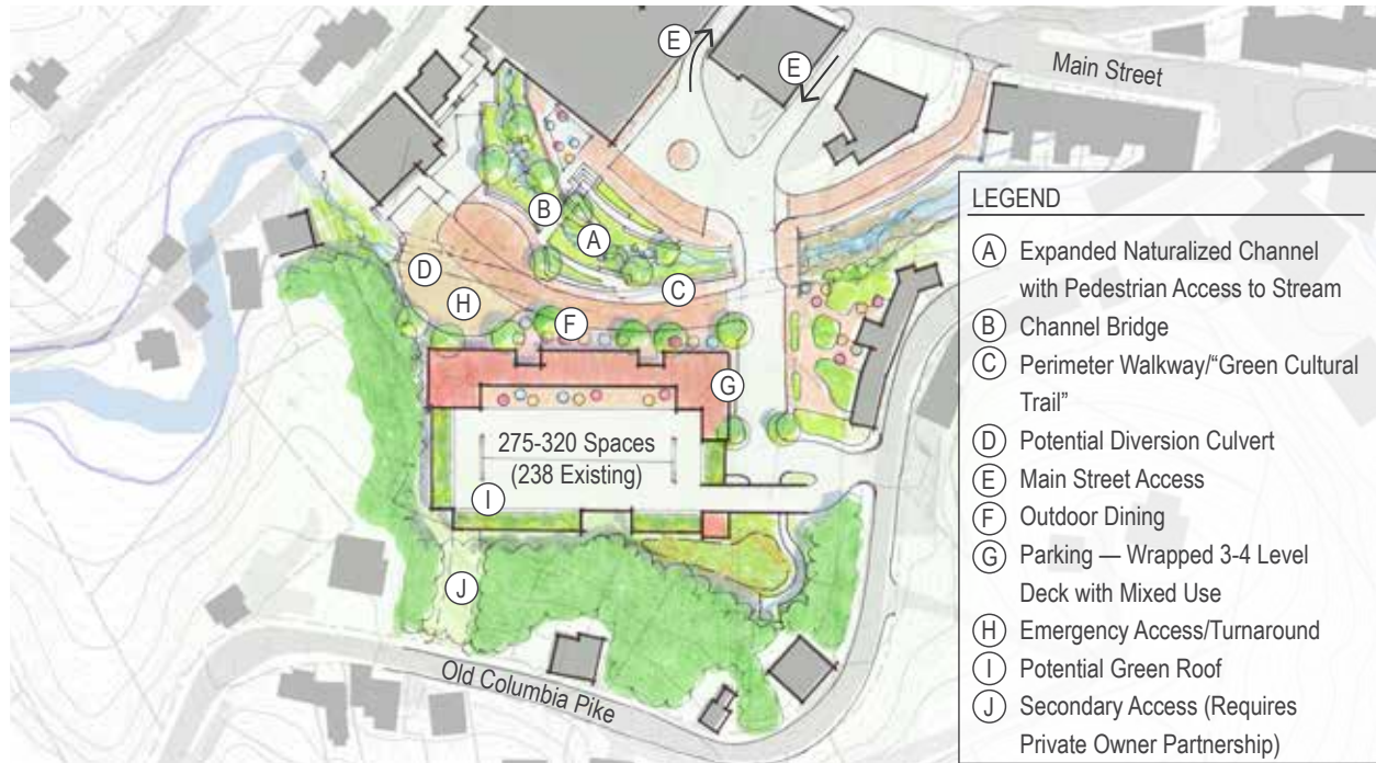
Figure 167: Parking Garage with Green Roof Elements, Mixed Use Space and Activated Channel
