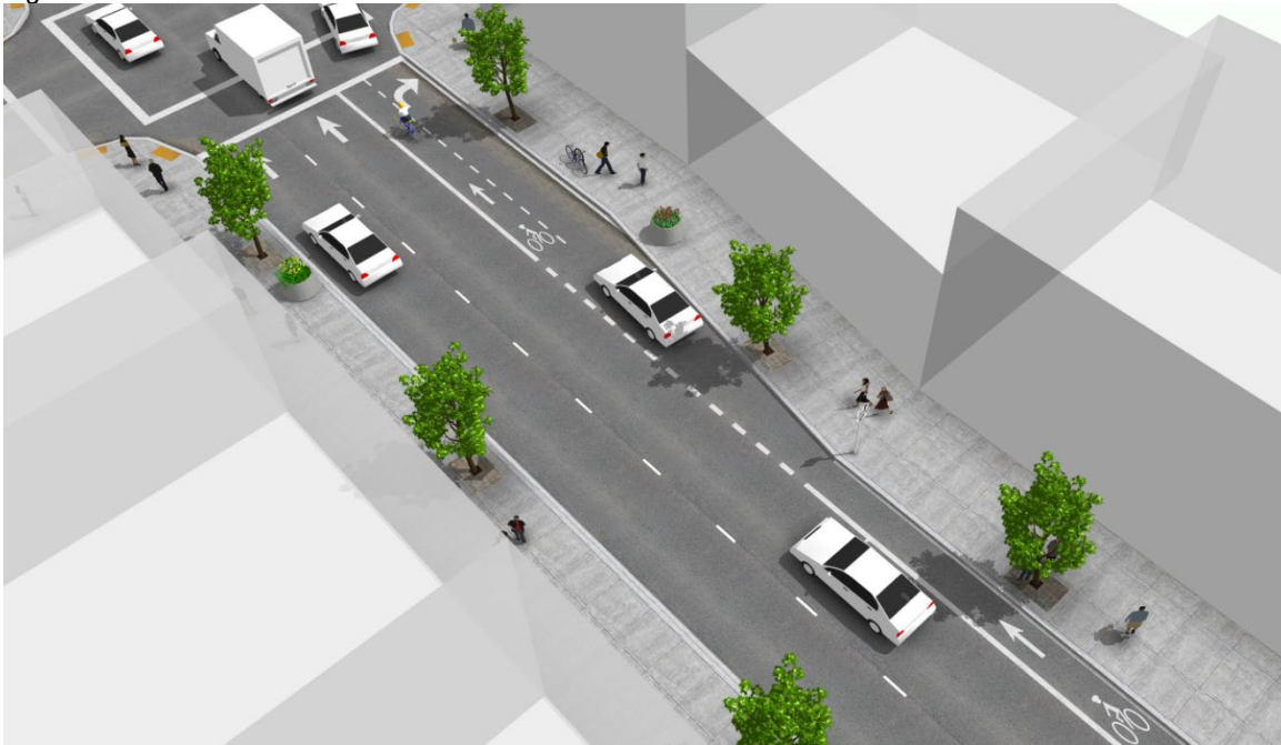
Figure 2-34. Combined Bike Lane/Turn Lane.
