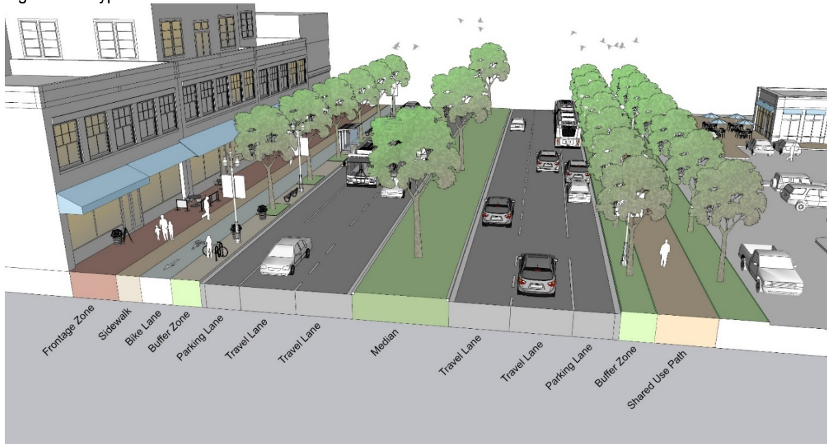
Figure 2-2. Typical Section Elements.
