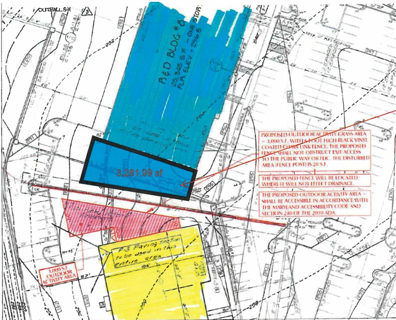
Make sure the fence foundation is not overlapping with 6" TAP and RCP
