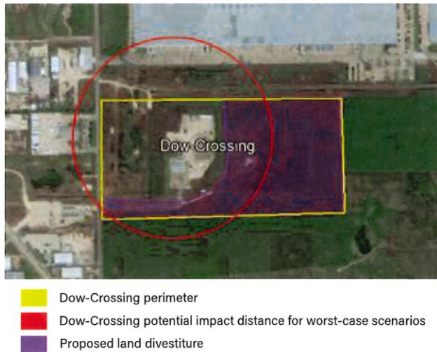
▲ Figure 3. An offer was received to purchase a portion of land within Dow-Crossing. Because the proposed land divestiture fell within the potential impact area, Dow declined the offer.
