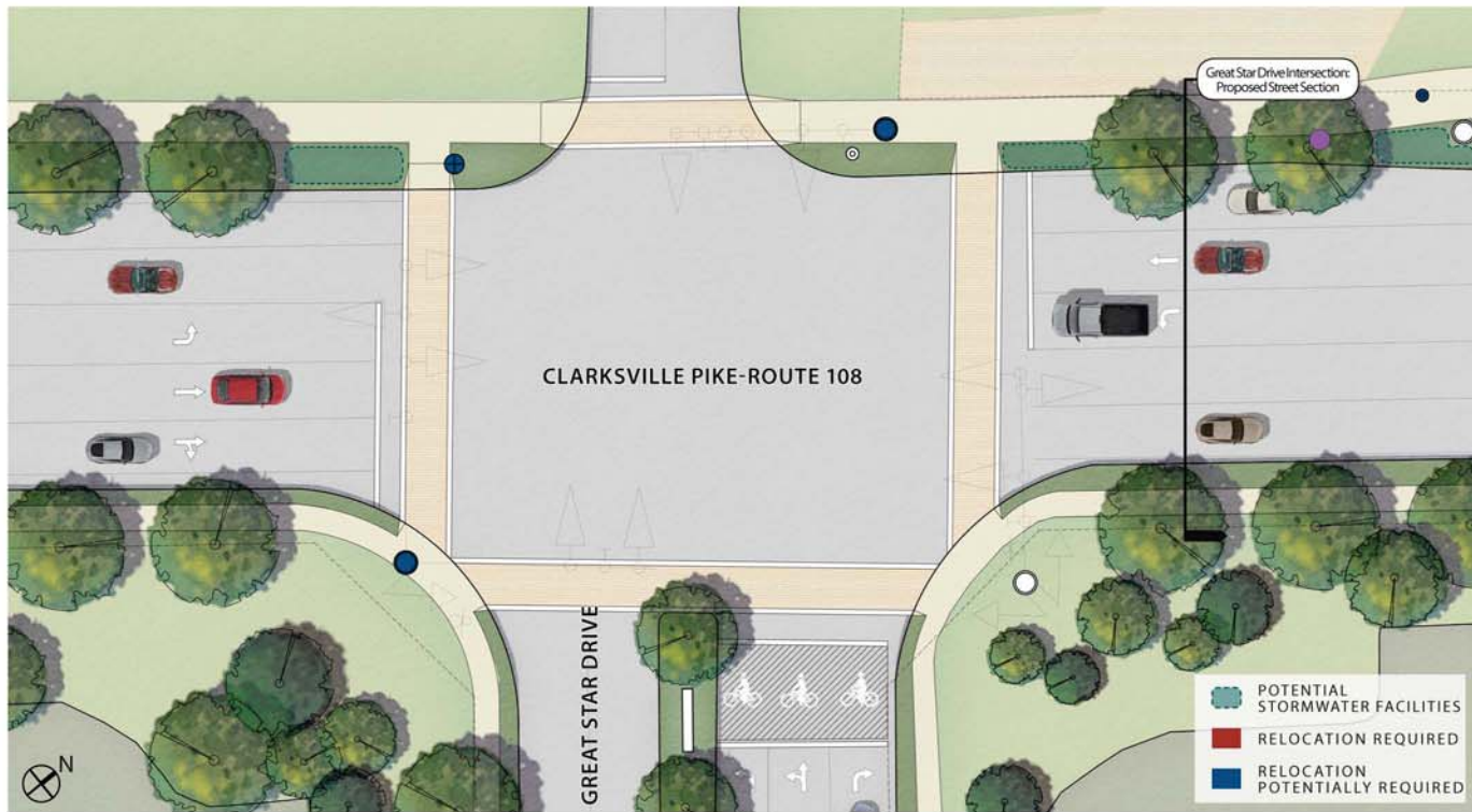
Proposed Streetscape: Streetscape improvements at Great Star Drive include crosswalks and ADA ramps, a continuous shared-use path along the western edge of Clarksville Pike, continuous sidewalks on the eastern edge and continuous planting strips and street trees on both sides. Bike accommodations along Great Star Drive at the intersection of Clarksville Pike are incorporated. Utility, signage and traffic signal poles may need to be relocated.
