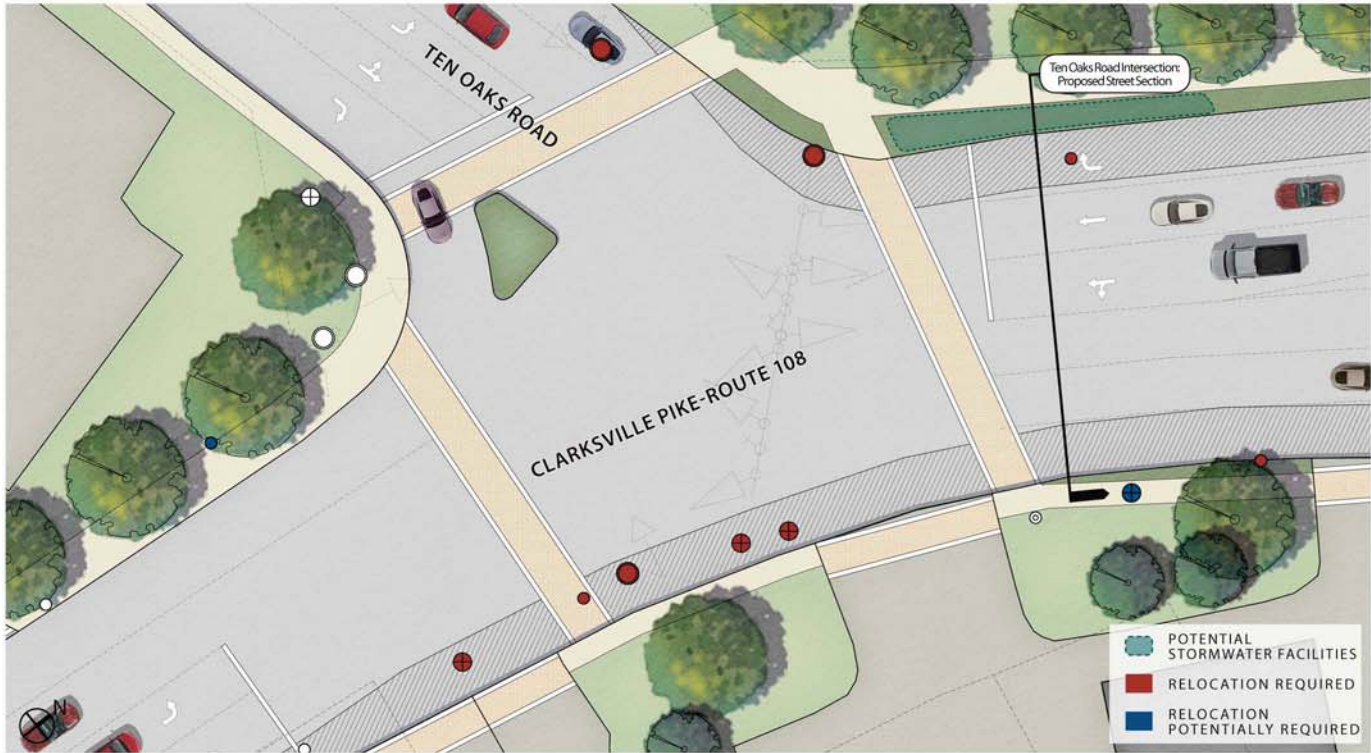
Proposed Streetscape: The long-term streetscape improvements at Ten Oaks Road include the integration of crosswalks and ADA ramps, a continuous shared-use path (west side only), continuous sidewalks and street trees. Existing utility, signage and traffic signal poles may need to be relocated in the future.
