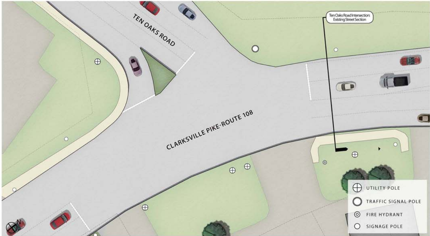
Existing Streetscape: The existing streetscape consists of intermittent sidewalks that do not connect. No ADA ramps or crosswalks exist in this portion of Clarksville Pike.
