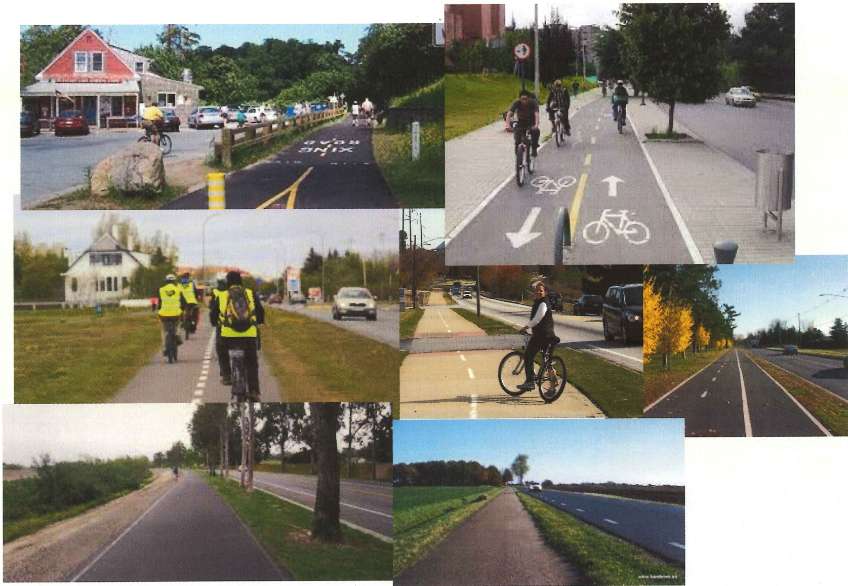
Images of “sidepath” bikeways with separating medians
